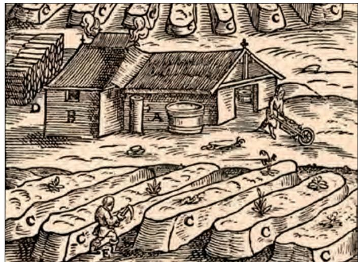
*A typical nitrary (Germany, c.1580) with leaching deposits (C) filled with decaying vegetable material mixed with manure. A worker collects effloresced saltpetre from deposits, transporting it then to be concentrated in the factory (B) boilers. (Source: <https://en.wikipedia.org/wiki/Nitrary#/media/File:Salnitrrera.jpg>)*
