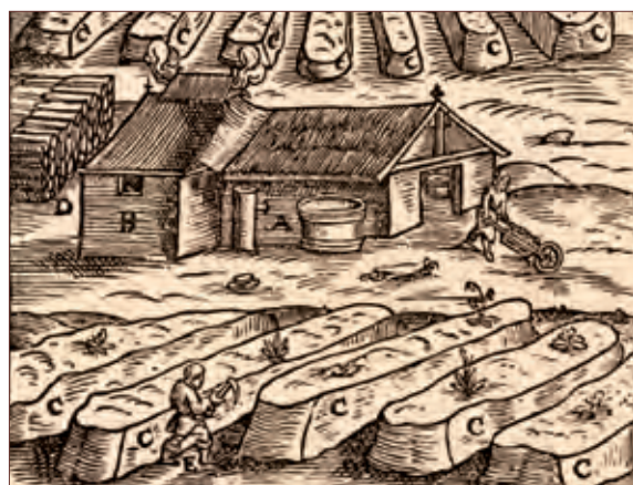
A typical nitrary (Germany, c.1580) with leaching deposits (C) filled with decaying vegetable material mixed with manure. A worker collects effloresced saltpetre from deposits, transporting it then to be concentrated in the factory (B) boilers. (Source: https://en.wikipedia.org/wiki/Nitrary#/media/File:Salmitrera.jpg )
